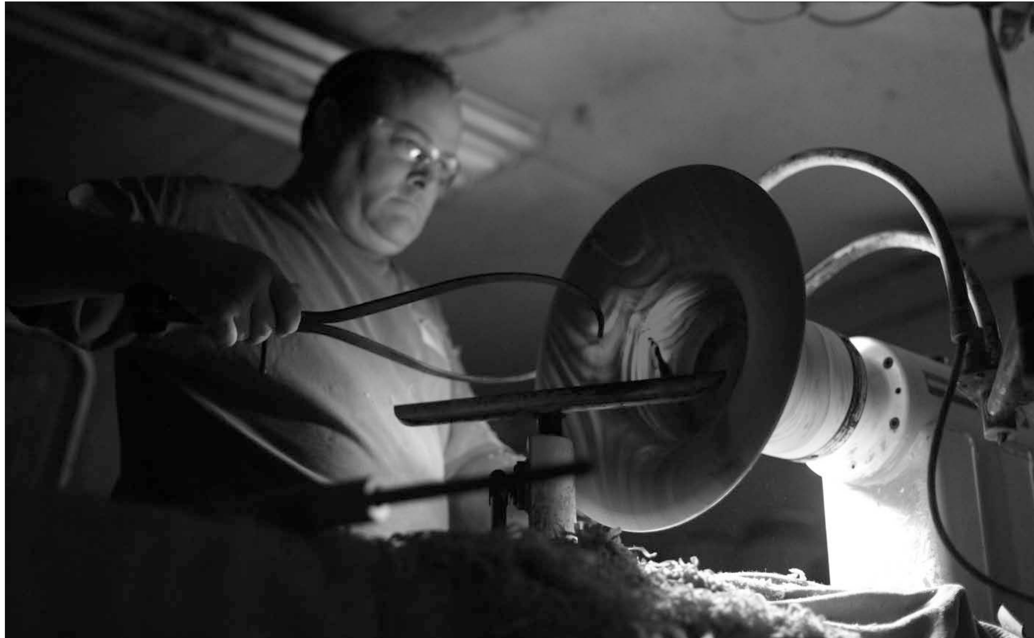
ABOVE • In the final stages of production, Chris Ramsey shines a light through the thin wood of a custom hat to help him ensure that it is not becoming too thin.
