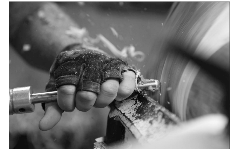
RIGHT • Using a lathe, professional wood turner Chris Ramsey carves a cowboy hat from single 135-pound piece of cherry.
